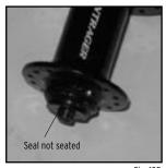
smooth transition from seal to sealing surface. An improperly installed seal (Fig. 10B) will allow rapid contamination of the bearings.
